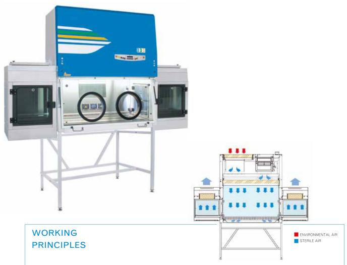
Ambient air is pulled from the H14 HEPA/ULPA filter inlet positioned on top of the isolator and then pressurized downwards towards the work surface prior to be H14 HEPA/ULPA filtered by the main filter. The air is partially re-circulated and partially exhausted via side transfer hatches before being washed again by virtue of a double set of H14 HEPA/ULPA filters fitted inside the hatches.
