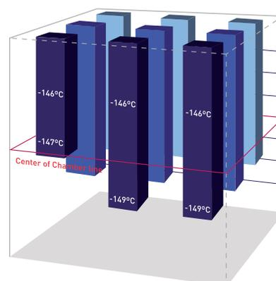
Comparison of temperature distribution in a liquid nitrogen freezer (vapour phase) and our MDF-C2156VAN mechanically refrigerated **Cryogenic** Freezer. The graph shows temperatures at different locations within the chamber. This data demonstrates that 100% of the MDF-C2156VAN storage space maintains uniform storage temperatures safely below -130°C, while temperature in the LN<sub>2</sub> vapour system is dependent on storage location.
