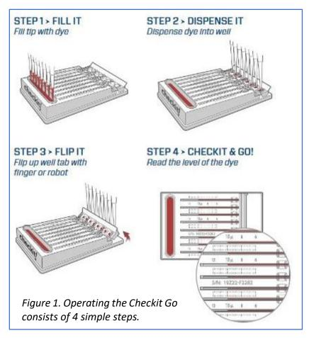
compared alongside graduations, as with a bulb thermometer.
