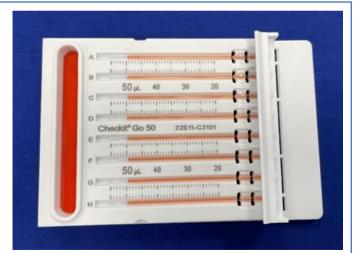
Figure 2. A Checkit Go ready for step 4. To read the actual volumes dispensed, simply compare the menisci against the graduations alongside the capillaries.
