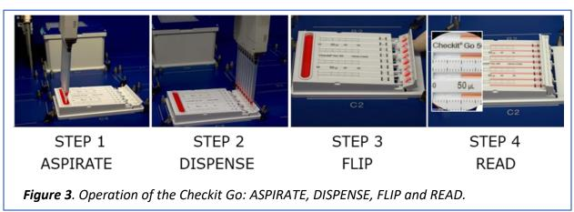
The Checkit Go cartridge has the same footprint of a standard microplate, so it fits in all automated liquid handlers that accommodate 96 or 384 well plates. Labware definitions and liquid classes are available for many manufacturers on our website, at, <a href="https://www.nextadvance.com/checkit-qo/resources">www.nextadvance.com/checkit-qo/resources</a>.
