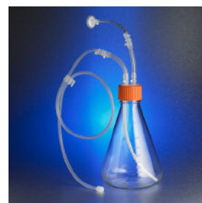
11440 Erlenmeyer Flask with attachment for Luer syringe at the vent.
