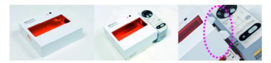
Step 4:Make sure the power safety buttons of *Mupid<sup>TM</sup> One* have been pressed by the 2 hooks on sidewall of the MUPID<sup>TM</sup> LED Illuminator
