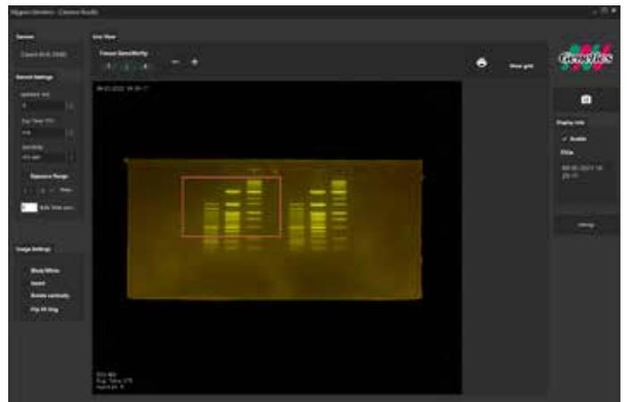
With the imaging software of the FAS-DIGI PRO you can control all necessary parameters of the camera to analyze and optimize any gel image. These four settings will provide the highest quality images for DNA gels: aperture, exposure time, sensitivity and focus.
