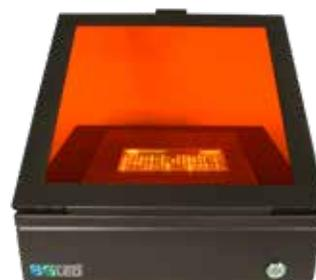
Using safe light, it becomes extremely simple to cut your DNA fragment out of gels. You don't need to wear protective eyewear, or worry about DNA degradation.
