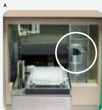
Instrument setup and performance tracking. A , onboard QC beads for hands-free QC process; B , QC Trending Report and ZE5-EYE Report for instrument performance monitoring.
