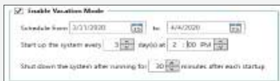
Set up the Vacation Mode for automatic Startup and Shutdown during prolonged instrument downtime.
