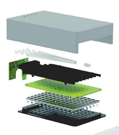
The Absorbance 96 is the first microplate reader on the market to contain 96 individual detection units. This means that all wells can be read simultaneously allowing for extremely fast photometric measurements. Without the need to scan across multiple wells, the Absorbance 96 has no moving parts. In combination with long-life LEDs, this solid-state design provides a maintenance-free user experience and ensures reliable, high quality results.
