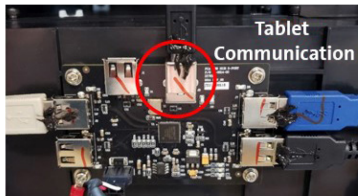
Figure 3. USB hub with the tablet communication cable connection indicated.
