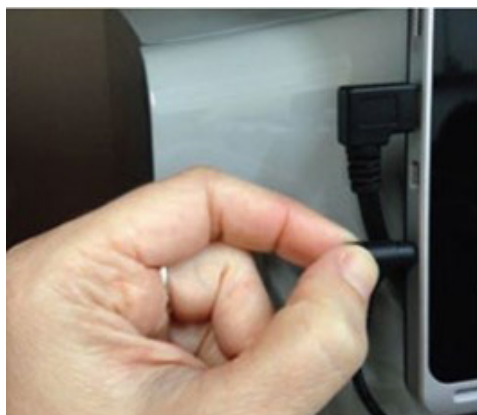
Figure 5. Power and communication cable connections to the replacement tablet.
