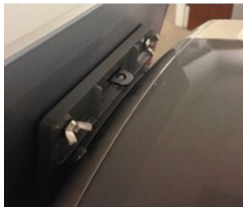
Figure 4. Wing nuts securing the tablet to the mounting bracket on the front of the system.
